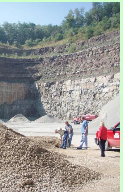
Sampling from a stockpile should always be done using a loader to separate out small sampling pile(s).
