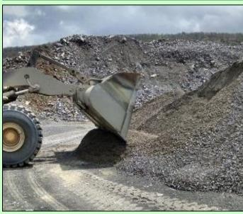
Mentally divide the flat sampling pad into four quadrants and sample equally from each quadrant. Avoid sampling within 1 foot of the pad edge and take care to avoid previous shovel holes.
