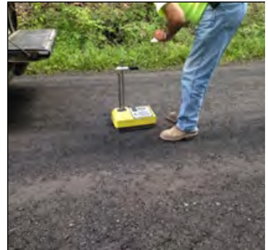
Figure 17. Compaction Testing with Nuclear Density Gauge
