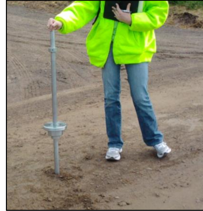
Figure 5.9: The dynamic cone penetrometer pictured here is used to measure road surface strength.
