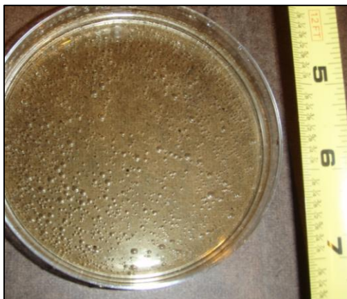
Figure 2.4: One of the petri dishes used to capture and suspend raindrops in order to measure their size.
