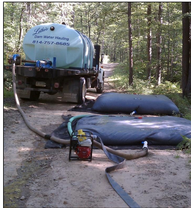
Figure 2.2: A water truck fills two 1,250 gallon collapsible bladders with water on site “T”.
