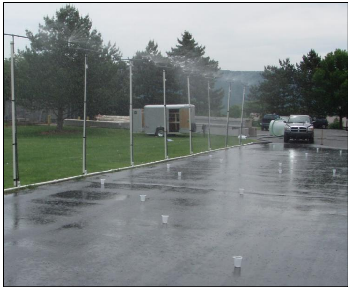
Figure 2.3: Rainfall collection jars were used to measure and calibrate the rainfall simulator.
