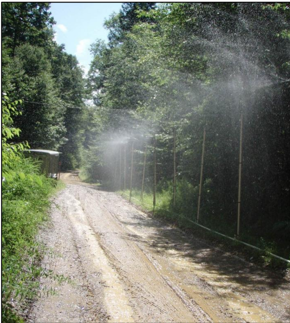
Figure 2.1: RainMaker being run on road Segment “R” as part of this study.
