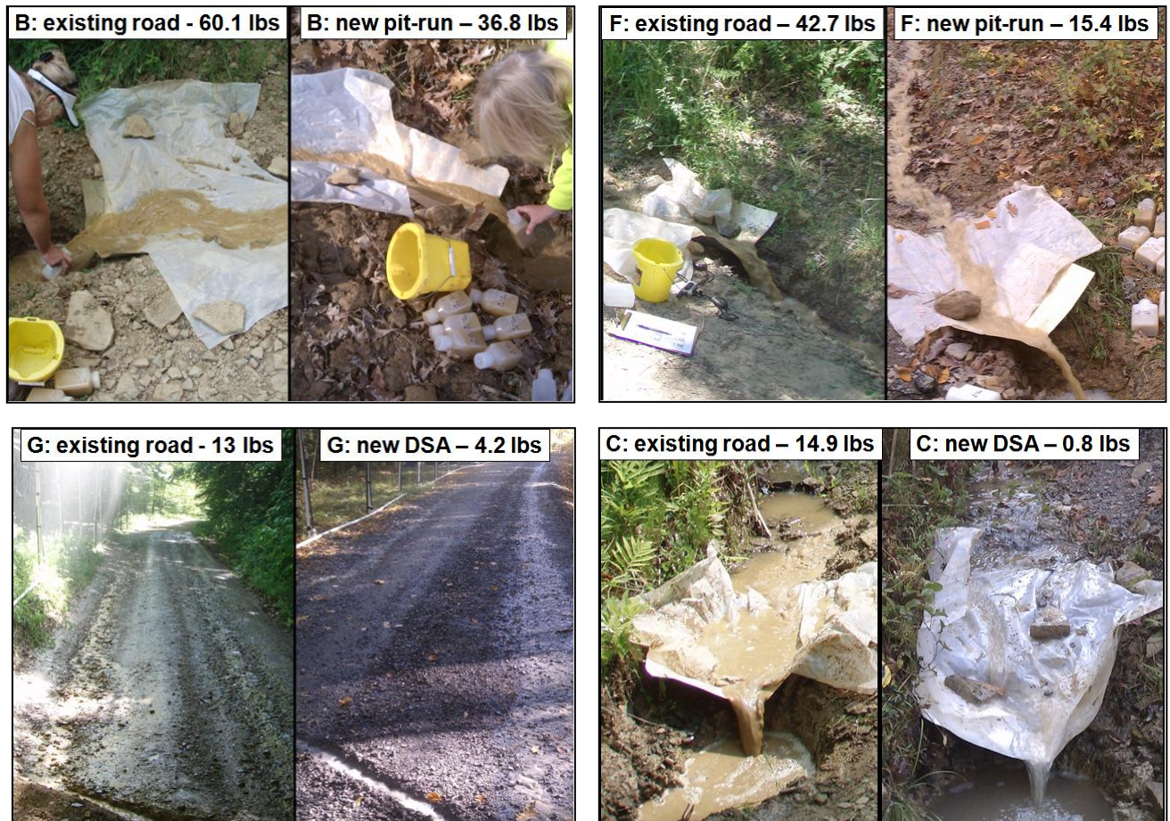
Figure 5.16: Visual comparison of the four sites in exiting condition during testing in 2010 and with new aggregate during testing in 2011. Average sediment production for three runs is included on each photo.
