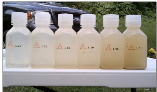
Figure 5.2: Runoff samples from site A are arranged by time, with T=1 on the right, through T=30 on the left.
