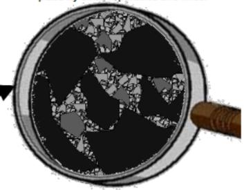
The above illustration shows how the various size components of DSA lock together compacted to produce the most dense and durable aggregate surface possible. The specification is well graded from large pieces that give support, all the way down to the "fines", rock particles less than 1/300th of an inch. This well graded mix including fines allows DSA to achieve a very high density. The box to the left illustrates the actual sizes of a "midline" or average DSA specification.
