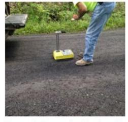
Figure 4: Compaction Testing with Nuclear Density Gauge
