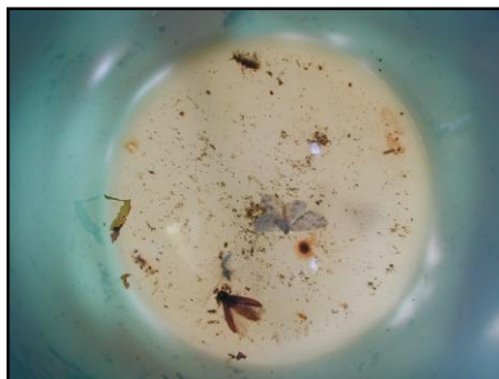
Figure 10. Contents of a dust fall jar as it was collected in the field.
