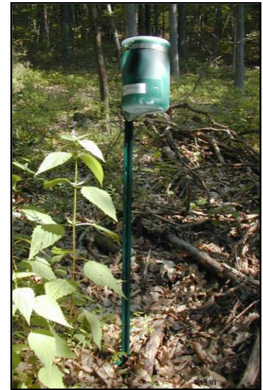
Figure 7. Typical dust fall jar placement.
