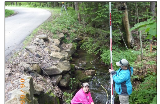
Conducting a longitudinal profile is essential to making the best structure selection.
