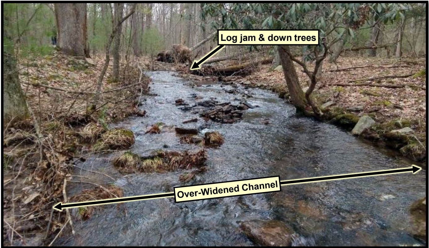
This photo shows a stream section with locations to avoid when measuring bankfull . In the foreground, the channel is over-widened and there is noticeable vegetation in the stream. Upstream there is a log jam and downed trees impacting the stream channel. Remember to be flexible when locating the best representation of the natural channel.
