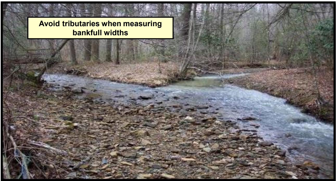
Additional water sources such as tributaries, springs, or tile drains add additional flow and change the bankfull width. If additional water enters above the crossing, then measurements should be taken downstream of the crossing. If additional water enters below the crossing, then measurements should be taken upstream of the crossing. Bankfull measurements of tributaries cannot simply be “added” to get an accurate bankfull width of the combined channel.
