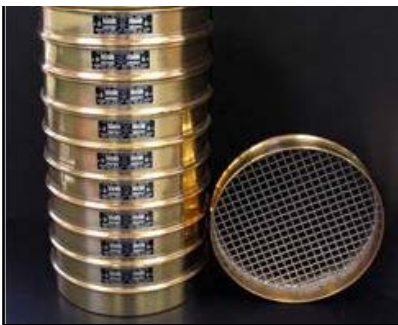
Aggregate sieves used to separate material by size (gradation). 1/2 inch or 12.5mm sieve visible on right.
