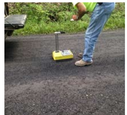
Figure 4 - Compaction Testing with Nuclear Density Gauge
